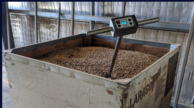
Top: John Fielke with 2 metre moisture spear ready to insert into stockpile of almonds.
