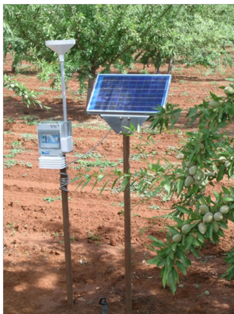
Figure 7: The Model T MetStation™, is both an automatic weather station (AWS) and a disease predictor for almond rust. The solar cell powers a mobile phone attachment allowing easy access to the data from a remote location.
