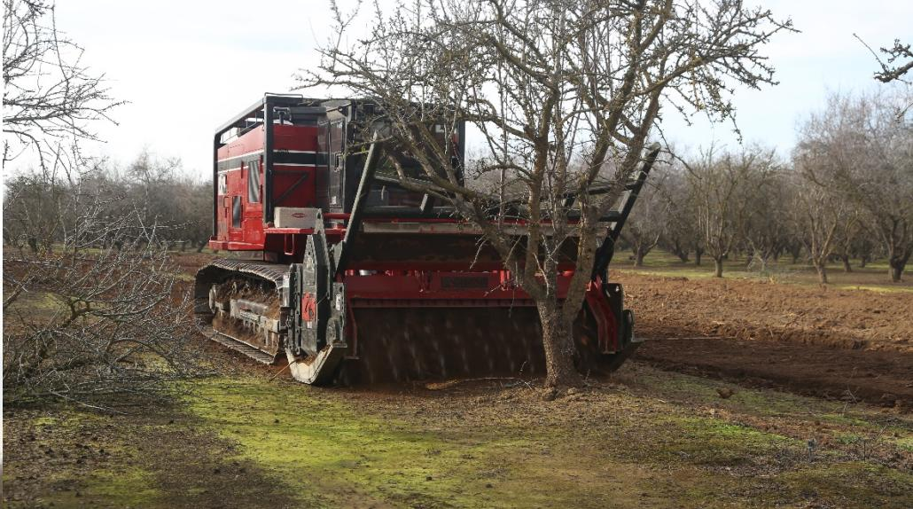
Then Iron Wolf goes in reverse and incorporates the wood into the ground. Just one 50 ton machine that costs \$1,500 acre to operate. Can do ~2 acres per day.
