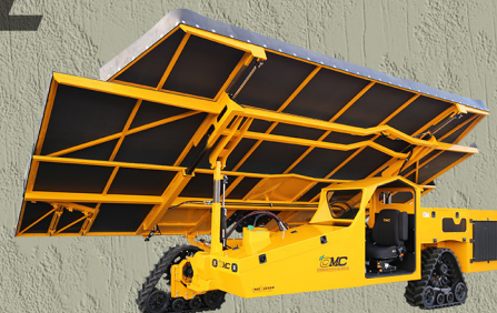
Catchall X 2-PIECE SHAKER/RECEIVER HARVESTER 3,8L Cummins Stage V turbo diesel engines New R-5 Magnum shaker head Optional tracked drive
