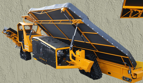
Catchall X 2-PIECE SHAKER/RECEIVER HARVESTER 3,8L Cummins Stage V turbo diesel engines New R-5 Magnum shaker head Optional tracked drive
