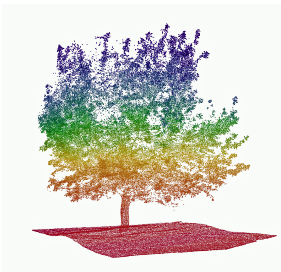
Figure 1. Low resolution LiDAR point cloud (15 percent of datapoints) of a three-year old Nonpareil almond tree. Canopy light interception and distribution can be determined from the full resolution image by simulating and tracing the sun’s rays through the canopy. Colours show the tree height above ground level.
