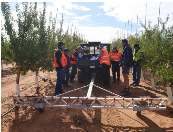
Figure 4. Members of the Crop Reference Group examining the SARDI Mobile Orchard Phenotyping Platform (MOPP) used to collect light interception and tree dimension data from trees in the Super High Density trial block at the ABA orchard in Loxton North. Image supplied by Ben Wiblin.
