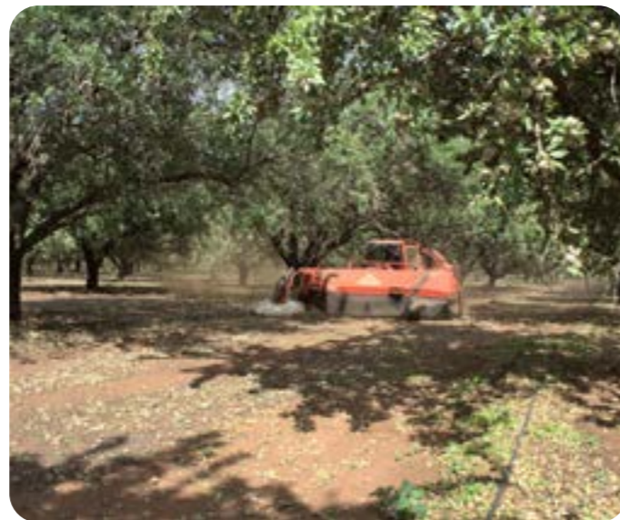
Figure 3. A first sweep (and blow) removes nuts from the tree base and drip-line so they don't get wet from irrigation.
