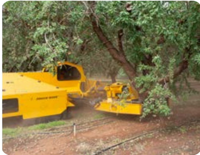
Figure 1. A harvest machine is used to shake fruit off trees once they have reached maturity and have sufficient moisture and weight to assist with shaking. If rain is imminent, do not shake. The best place for almonds is to remain on the tree where there is good air circulation around the fruit.
