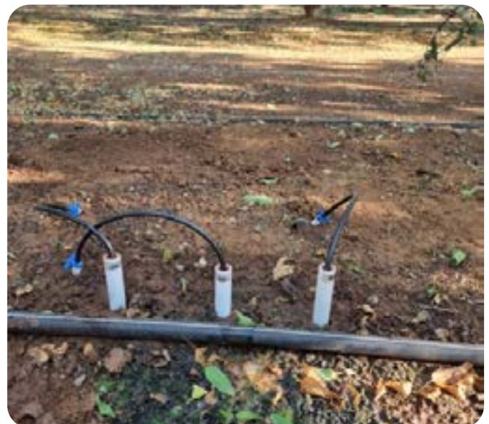
Figure 2: SWEs installed in a cluster or nest at three depths 30cm, 60cm and 90cm can monitor the movement of soil water and nutrients into the soil profile.
