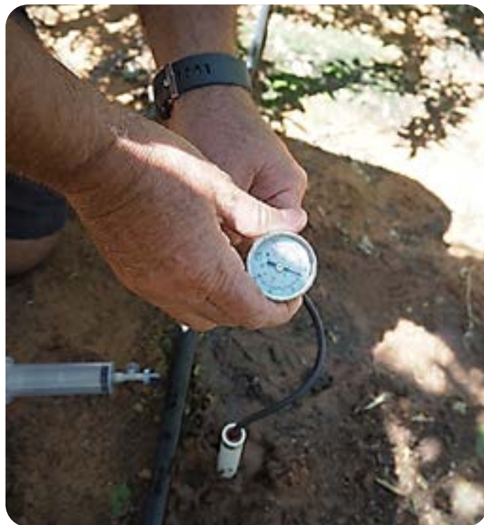
Figure 6: The gauge shows the ideal vacuum for the SWE (-50 to -60 kPa). Heavier soils may need priming to -70kPa in order to extract soil water.
