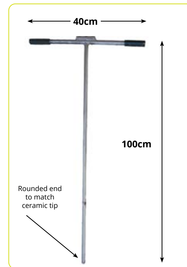
Figure 5: T-bar steel auger dimensions.
