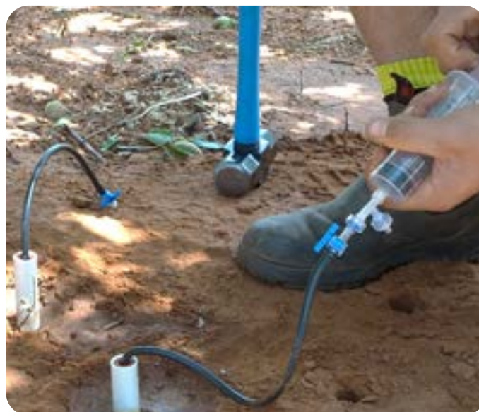
Figure 4: Close-up of syringe attached to the SWE. The stopcock is 'open' ready to prime the SWE. After priming the blue tap would need to be closed before disconnecting the syringe. The syringe and tube is now primed i.e. at a negative or suction pressure needed to draw water from the soil profile.
