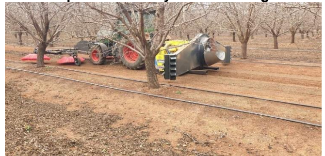
Figure 4. sweeping, flail mulching and blowing all in one pass to destroy overwintering
