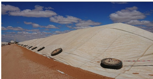
Figure 3. Stockpile that has been correctly sealed ready for fumigation.
