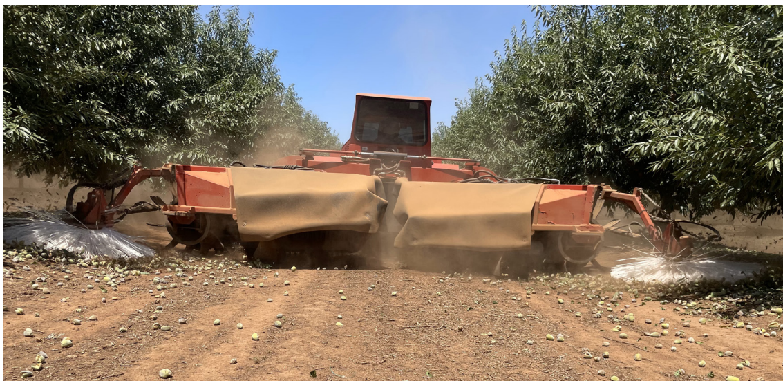
Image 1. A level sweeper with well positioned brushes creating minimal dust.
