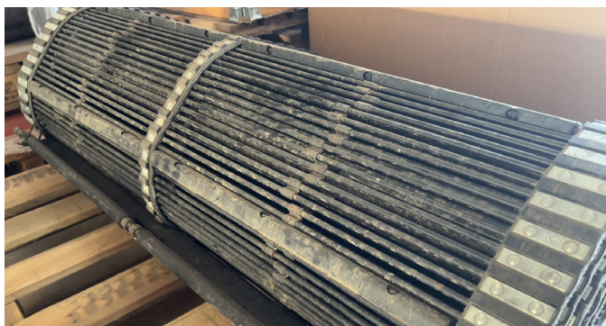
Image 2. Modern cleaning chains (twin rod) on harvesters enable dirt to drop back onto the ground.
